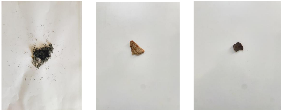
Plate 11: Bioplastic sample after flame test
