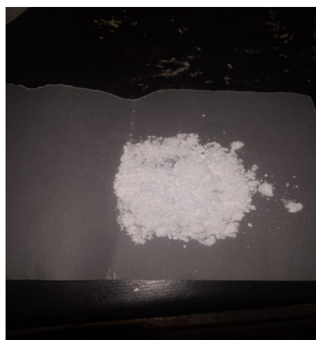
\text{Al}_2\text{O}_3 nanopowder formed after calcination
