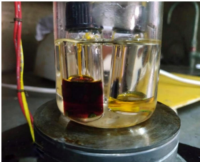
Figure 2.5 - Growth of Single Crystal in oil bath
